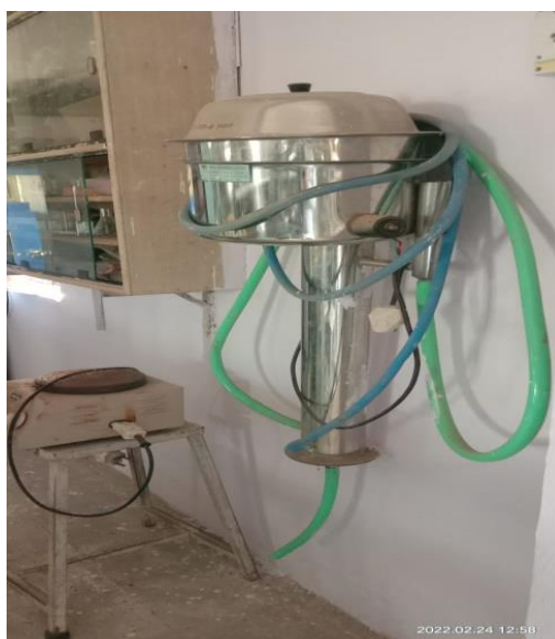
Water Distillation Unit
